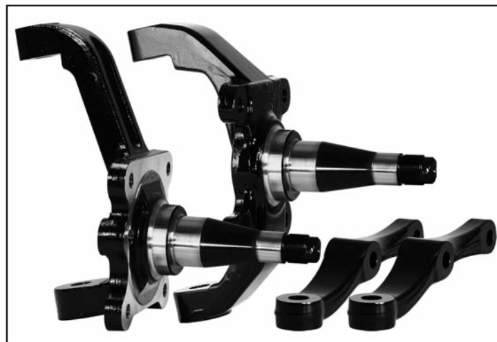
Standard Height Spindle Shown Left, 2" Drop Spindle Shown Right with Detached Steering Arms (one per spindle)
